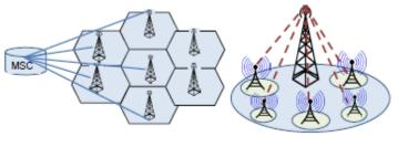
a. Base station-centric network b. Small cell network
